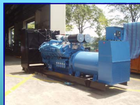
CUMMINS Powered Genset
