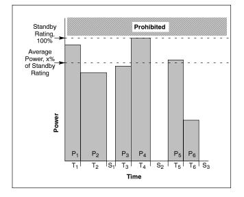
\* Waukesha-powered models may run up to 3500 hours per year while maintaining a standby rating. KM-powered models are limited to 100 hours per year.
