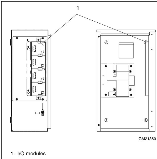
**Figure 6-10** Typical I/O Module Locations (welded enclosures)
