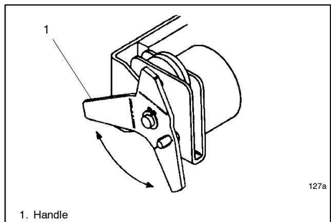
**Figure 2-7** Manual Operation Handle, 30-200 Amp Open-Transition Switches
