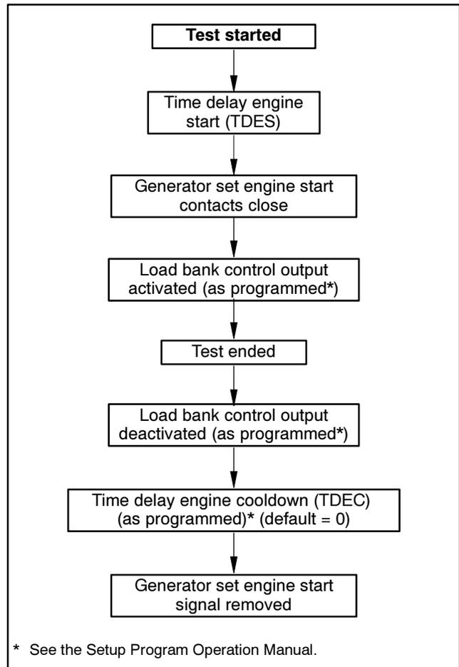
**Figure 4-4** Test Without Load Sequence
