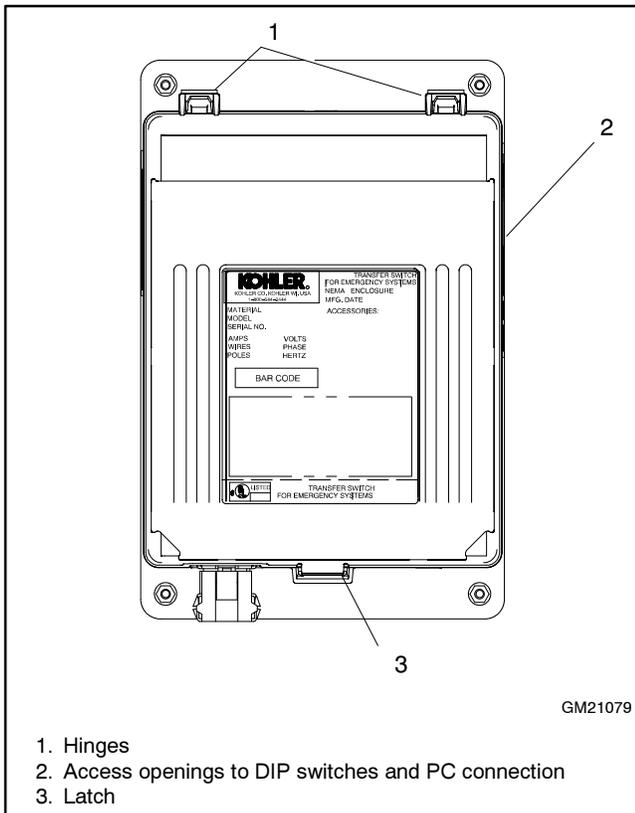
**Figure 3-5** Controller Housing
