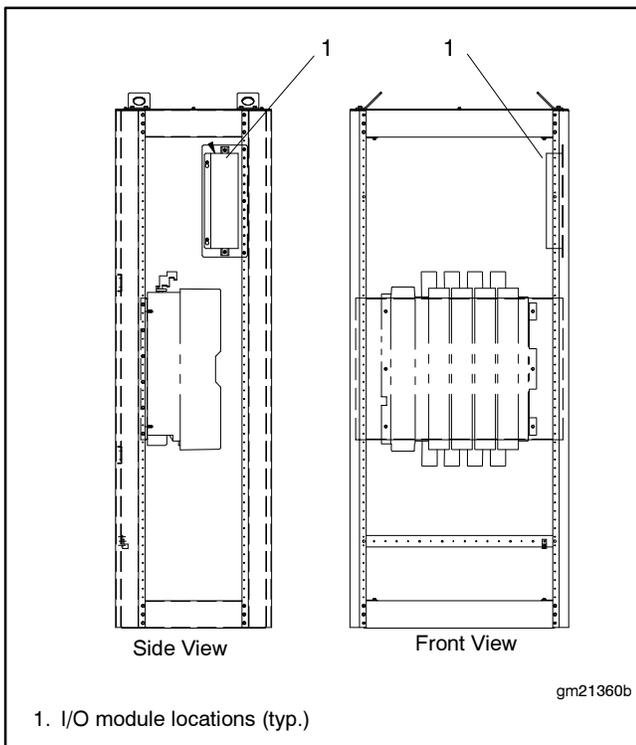
**Figure 6-11** Typical I/O Module Locations (framework enclosures)
