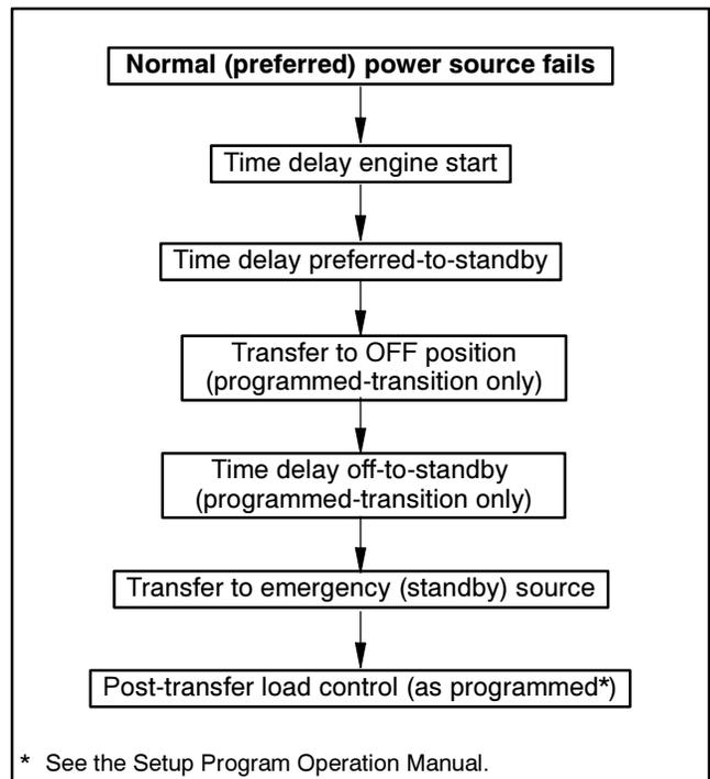
**Figure 4-1** ATS Sequence of Operation, Transfer to Emergency (standby source)
