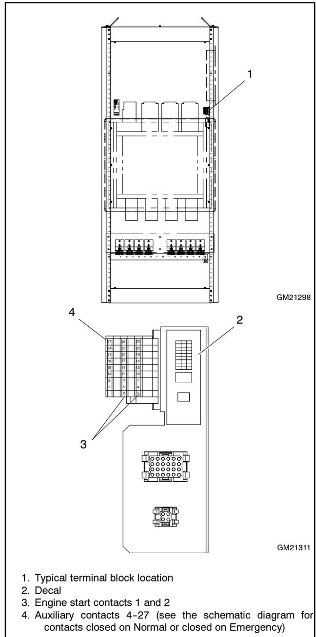
**Figure 2-23** Engine Start and Auxiliary Contact Terminal Block, Programmed-Transition Models and 600-4000 Amp Open-Transition Models
