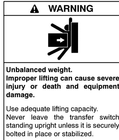
See Figure 2-1 through Figure 2-4 or the dimensional drawing for the weight of the transfer switch. Use a spreader bar to lift the transfer switch. Attach the bar only to the enclosure's mounting holes or lifting brackets; do not lift the unit any other way. Close and latch the enclosure door before moving the unit.
