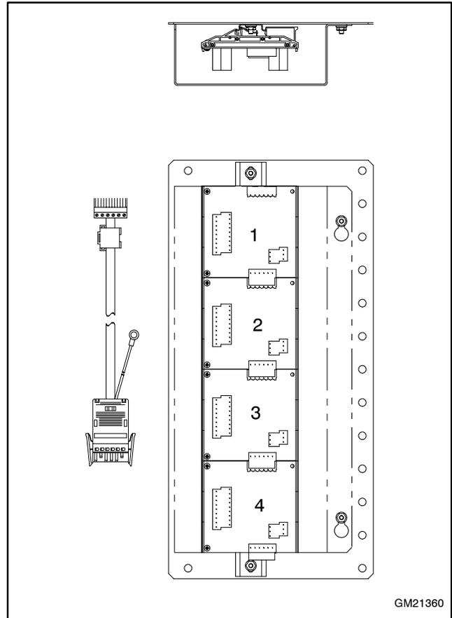
**Figure 6-9** Input/Output Modules and Harness (cover is shown transparent to show detail)
