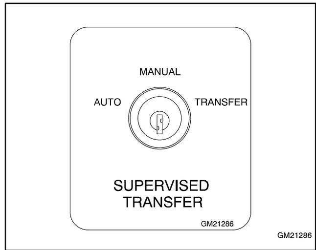
**Figure 6-4** Supervised Transfer Control Switch
