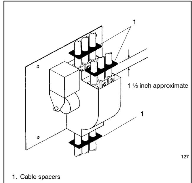
**Figure 2-16** Cable Spacers for 30-200 Amp Switches
