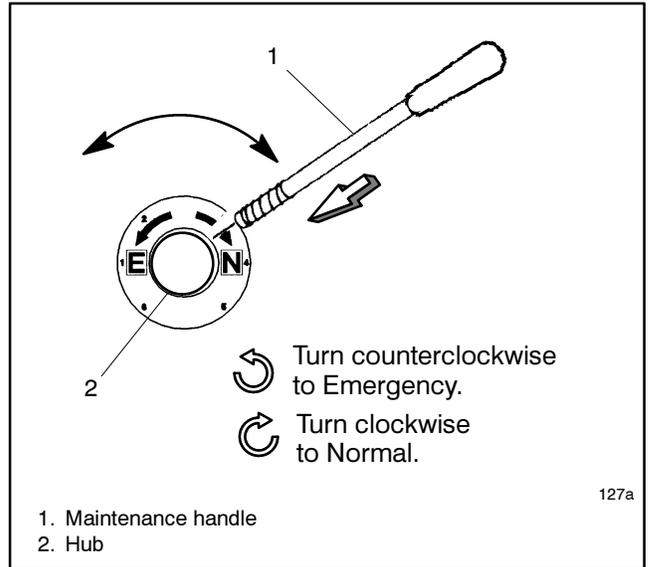
**Figure 2-11** Manual Operation, 1600-3000 Amp Switches
