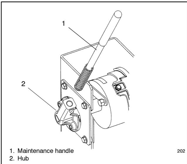
**Figure 2-10** Manual Operation, 600-1200 Amp Switches
