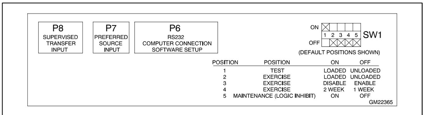
**Figure 3-8** Logic Assembly Decal Showing DIP Switch Settings
