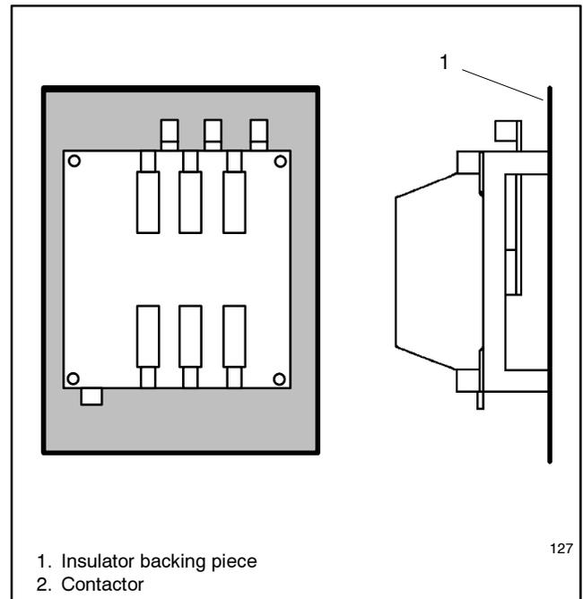
**Figure 2-17** Insulator for 225-400 Amp Switches
