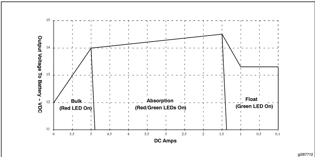
Figure 6-25 Charging Method, 12 VDC, 6 A Configuration
