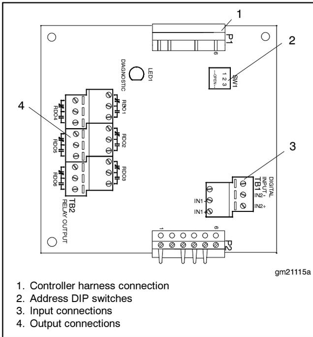
**Figure 6-14** I/O Module Input and Output Connections
