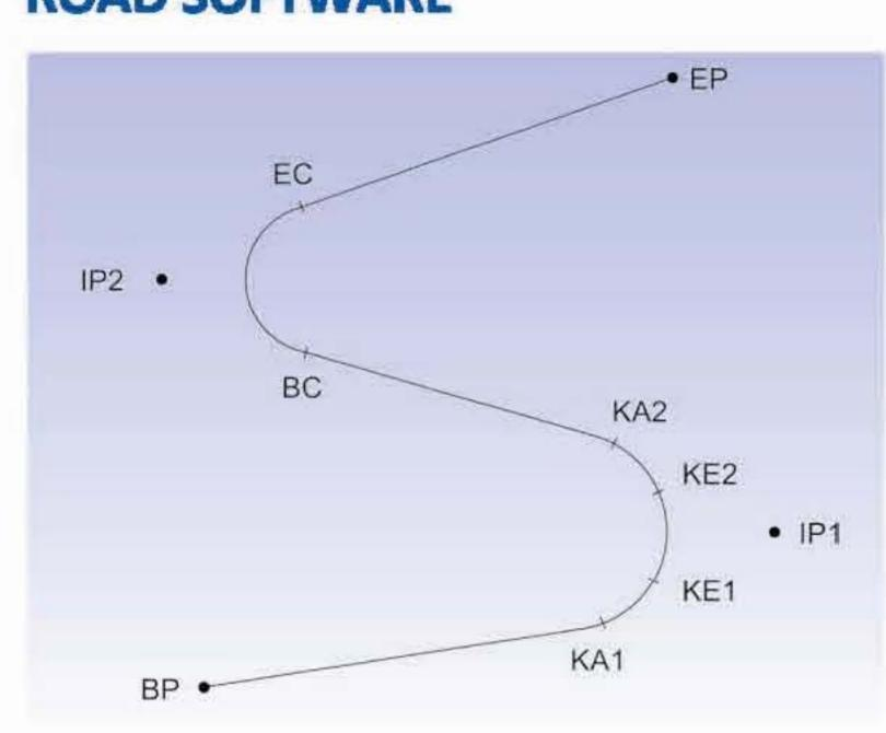
The on-board ROAD software satisfy your massive application measurement by automatically calculating complicated spiral curve and a long distance route by defining only the required points (start point, terminal point or curvilinear point) according to your needs.
