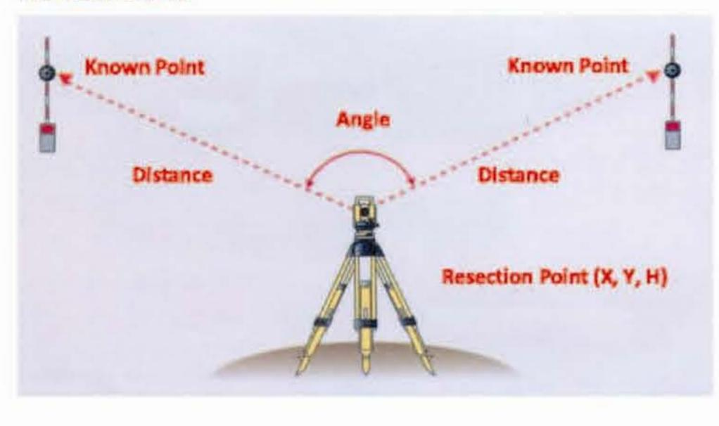
TKS-202 Total Station can determine the azimuth and coordinates with certain known points. This function is especially useful if the coordinates of the specific instrument station is unknown. Elevated station from two known reference points can also be calculated, with each deviation of multiple reference points being displayed.
