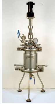
4-liter, 6" jacketed Benchtop Nutsche with motorized up/down cake agitator (& special upside-down hanging arms)
