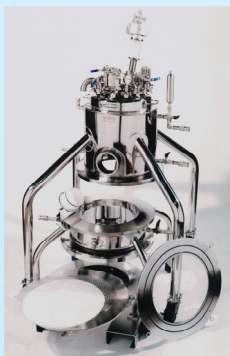
37 gallon, 18" 3-piece cake retention type, with jacket, 800 Mixer with air motor, side access port, 8 legs
