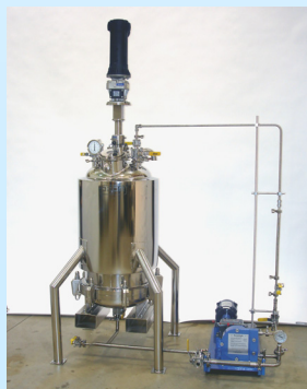
37 gallon, 18" unit with non-removable top head, jacket, 800 Mixer with XP motor, recirculation pump system
