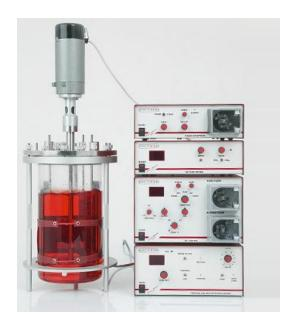
Each module, although totally independent, can stack together to create an extremely neat, combined unit with inter-linking power cables.
