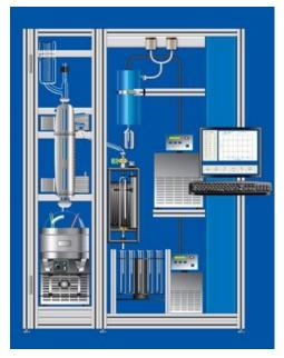
**Easy to Use**: PC control automates D2892 and D5236 crude oil distillations from beginning to end. New and experienced operators will find this system simple to use. The software steps you through D2892 and D5236 distillations.
