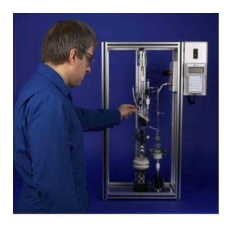
**Easy to Use:** PC control automates the mini crude oil distillation from beginning to end. New and experienced operators will find this system simple to use. The software steps you through crude oil distillation process
