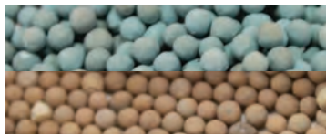
Moisture Adsorbent: Top: Full Capacity; Bottom: Depleted.
