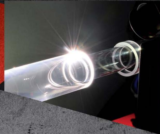
One important process step at the production of lamps is the cutting of glass tubes.
