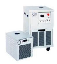
NRD-550 systems are equipped with digital temperature display, a coolant pressure gauge, a liquid level switch, and a flow/pressure adjustment valve. Heat removal capacities are dependent on the cooling water flow rate and on the process water flow rate. A variety of circulating pumps are available to match process requirements. Our engineers are happy to assist in selecting the proper circulating pump and heat exchange system.
