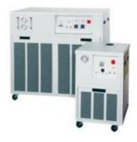
TKD-200/250 Chillers feature CFC-free refrigeration systems with compressor hot discharge gas bypass. Stability to  $\pm 0.5$ °C is maintained with our standard temperature controller with digital display of process/setpoint temperature. If still tighter stability is required, these chillers can be equipped with our microprocessor-based temperature controller that is stable to  $\pm 0.1$ °C.
