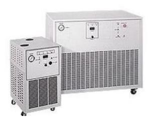
The TKD-100 Series Chillers' circulating pump and compressor motors are all thermally protected. Standard features include a liquid filled pressure gauge to indicate recirculating coolant outlet pressure and locking casters for easy portability. Filling of the coolant reservoir is easily accomplished through the top of the system. The quickly removable top and side panels simplify maintenance.
