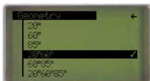
All selected angles measure at the same location and the results are displayed instantly – including Statistics, Difference or Pass/Fail. The micro-TRI-gloss has all functions of the new glossmeter generation readily at hand.
